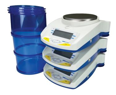
The Highland Portable Precision Balance is stackable, for efficient storing and transporting between classrooms.
