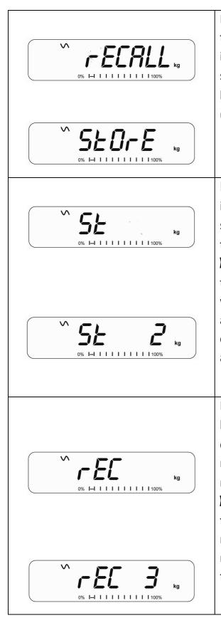
Press the [→Lim] key. If you are already in the check weighing mode the display will ask if you wish to store the current limits by showing **"StOFE"** or recall another set of limits by showing **"FECALL"**. The [→Lim] key can be used to toggle between **"StOFE"** and **"FECALL"**.
